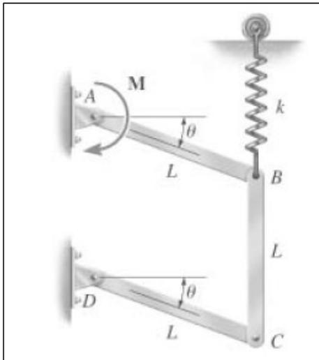
$$y_1 = \left(\frac{L}{2}\right)\sin(\theta) \quad \delta y_1 = \left(\frac{L}{2}\right)\cos(\theta)\delta\theta \quad y_2 = L\sin(\theta) \quad \delta y_2 = L\cos(\theta)\delta\theta$$
