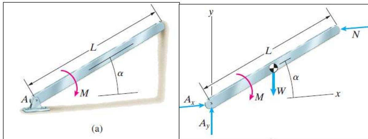
$$\begin{aligned}\Sigma F_x &= A_x - N = 0, \\ \Sigma F_y &= A_y - W = 0, \\ \Sigma M_{\text{point } A} &= NL \sin \alpha - W \frac{1}{2} L \cos \alpha - M = 0.\end{aligned}$$
