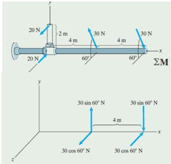
$$\begin{aligned}\Sigma \mathbf{M} &= 40\mathbf{i} + (30 \cos 60^\circ)(4)\mathbf{j} - (30 \sin 60^\circ)(4)\mathbf{k} \text{ (N-m)} \\ &= 40\mathbf{i} + 60\mathbf{j} - 104\mathbf{k} \text{ (N-m)}.\end{aligned}$$
