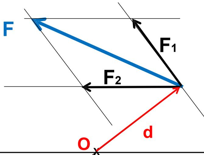
$$\bar{M}_{O,F} = \bar{d} \times \bar{F}_1 + \bar{d} \times \bar{F}_2$$
