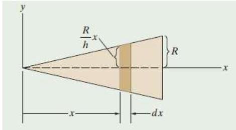
$$\bar{x} = \frac{\int_V x dV}{\int_V dV} = \frac{\int_0^h x \pi \left[ \left( \frac{R}{h} \right) x \right]^2}{\int_0^h \pi \left[ \left( \frac{R}{h} \right) x \right]^2 dx} = \frac{3}{4} h.$$
