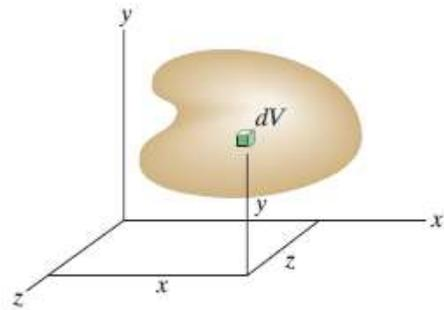
$$\bar{x} = \frac{\int_V x dV}{\int_V dV}, \quad \bar{y} = \frac{\int_V y dV}{\int_V dV}, \quad \bar{z} = \frac{\int_V z dV}{\int_V dV}.$$
