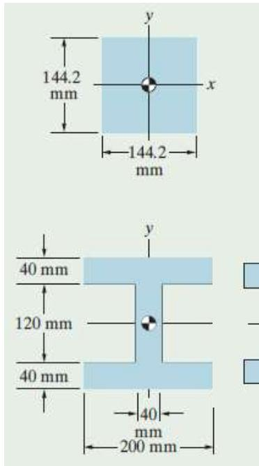
$$I_x = \frac{1}{12}(144.2 \text{ mm})(144.2 \text{ mm})^3 = 3.60 \times 10^7 \text{ mm}^4.$$
