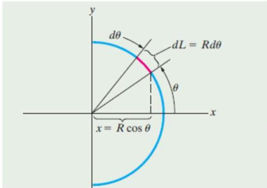
$$\bar{x} = \frac{\int_L x dL}{\int_L dL} = \frac{\int_{-\pi/2}^{\pi/2} (R \cos \theta) R d\theta}{\int_{-\pi/2}^{\pi/2} R d\theta} = \frac{R^2 [\sin \theta]_{-\pi/2}^{\pi/2}}{R [\theta]_{-\pi/2}^{\pi/2}} = \frac{2R}{\pi}$$
