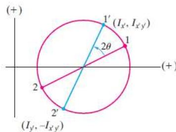
$$\sin \beta = \frac{I_{xy}}{R}, \quad \cos \beta = \frac{I_x - I_y}{2R}, \quad R = \sqrt{\left(\frac{I_x - I_y}{2}\right)^2 + (I_{xy})^2}$$
