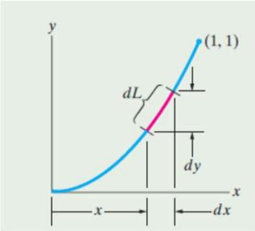
$$\bar{x} = \frac{\int_L x dL}{\int_L dL} = \frac{\int_0^1 x \sqrt{1 + 4x^2} dx}{\int_0^1 \sqrt{1 + 4x^2} dx} = 0.574.$$
