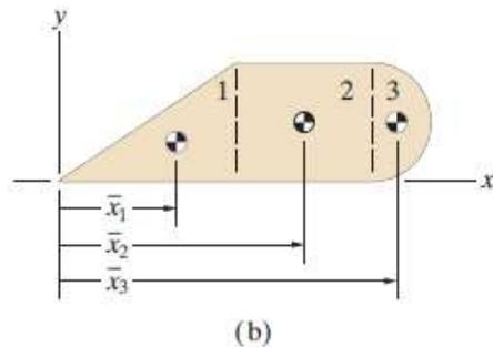
$$\bar{x}_1 = \frac{\int_{A_1} x dA}{\int_{A_1} dA}, \quad \int_{A_1} x dA = \bar{x}_1 A_1, \quad \bar{x} = \frac{\bar{x}_1 A_1 + \bar{x}_2 A_2 + \bar{x}_3 A_3}{A_1 + A_2 + A_3}$$
