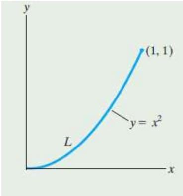
$$dL = \sqrt{dx^2 + dy^2} = \sqrt{1 + \left( \frac{dy}{dx} \right)^2} dx$$
