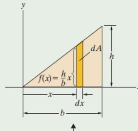
$$\left. \begin{aligned} (I_x)_{\text{strip}} &= \int_{\text{strip}} y^2 dA_s \\ &= \int_0^{f(x)} (y^2 dx) dy \\ &= \frac{1}{3} [f(x)]^3 dx. \end{aligned} \right\} \leftarrow$$
