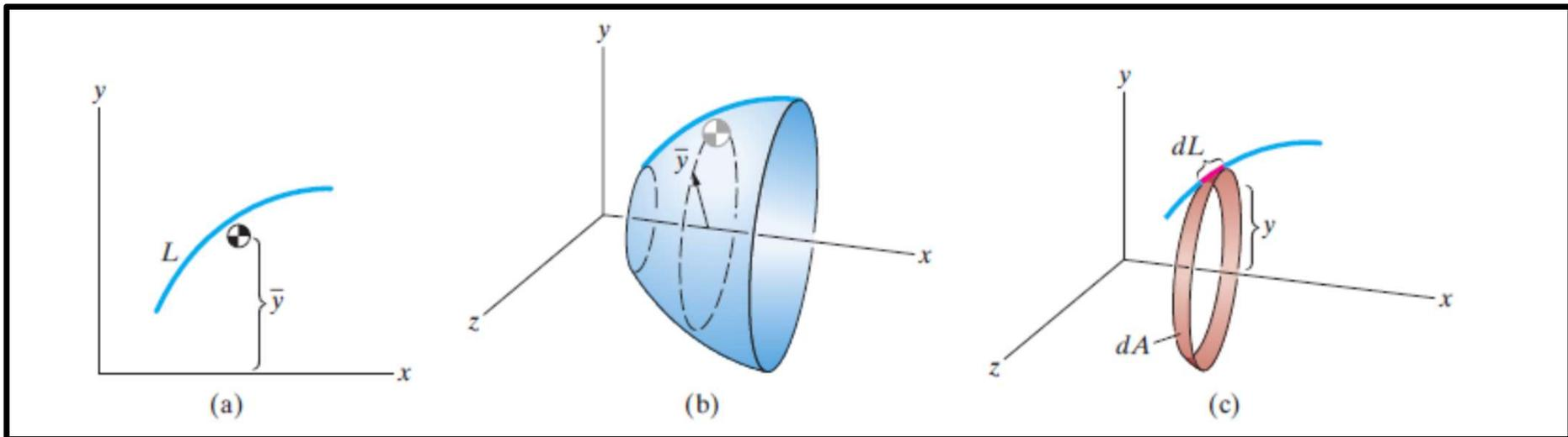
$$A = 2\pi \bar{y} L \qquad A = 2\pi \int_L y dL \qquad \bar{y} = \frac{\int_L y dL}{\int_L dL}, \qquad \int_L y dL = \bar{y} L$$
