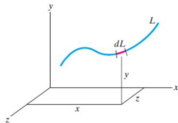
$$\bar{x} = \frac{\int_L x dL}{\int_L dL}, \quad \bar{y} = \frac{\int_L y dL}{\int_L dL}, \quad \bar{z} = \frac{\int_L z dL}{\int_L dL}.$$
