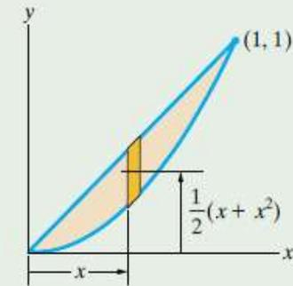
$$\bar{x} = \frac{\int_A x dA}{\int_A dA} = \frac{\int_0^1 x(x - x^2) dx}{\int_0^1 (x - x^2) dx} = \frac{\left[\frac{x^3}{3} - \frac{x^4}{4}\right]_0^1}{\left[\frac{x^2}{2} - \frac{x^3}{3}\right]_0^1} = \frac{1}{2}$$
