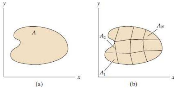
$$\bar{x} = \frac{\sum_i x_i A_i}{\sum_i A_i}, \quad \bar{y} = \frac{\sum_i y_i A_i}{\sum_i A_i}.$$
