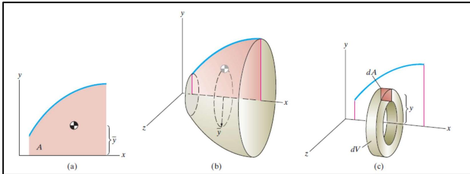
$$V = 2\pi\bar{y}A \qquad V = 2\pi \int_A y dA \qquad \bar{y} = \frac{\int_A y dA}{\int_A dA}, \qquad \int_A y dA = \bar{y}A.$$
