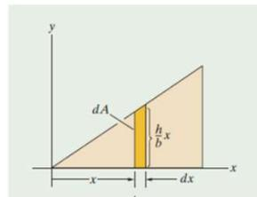
$$\bar{x} = \frac{\int_A x dA}{\int_A dA} = \frac{\int_0^b x \left(\frac{h}{b} x dx\right)}{\int_0^b \frac{h}{b} x dx} = \frac{\frac{h}{b} \left[\frac{x^3}{3}\right]_0^b}{\frac{h}{b} \left[\frac{x^2}{2}\right]_0^b} = \frac{2}{3}b.$$
