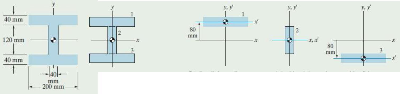
Determining the moments of inertia of the parts about the  $x$  axis.
