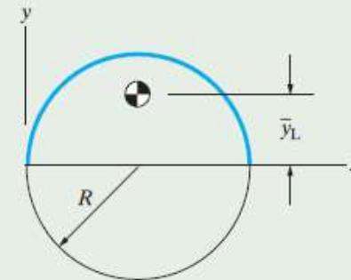
Revolving a semicircular line about the  $x$  axis.
