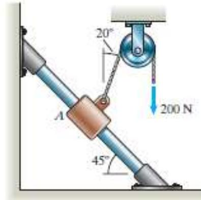
**Solution:** The pulley does not change the tension in the rope that passes over it. There is no friction between the slider and the bar.
