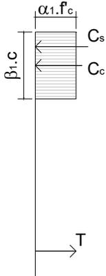
$T = f_y \cdot A_s = 42 \text{ kN/cm}^2 \cdot 19,64 \text{ cm}^2 = 824,88 \text{ kN}$
