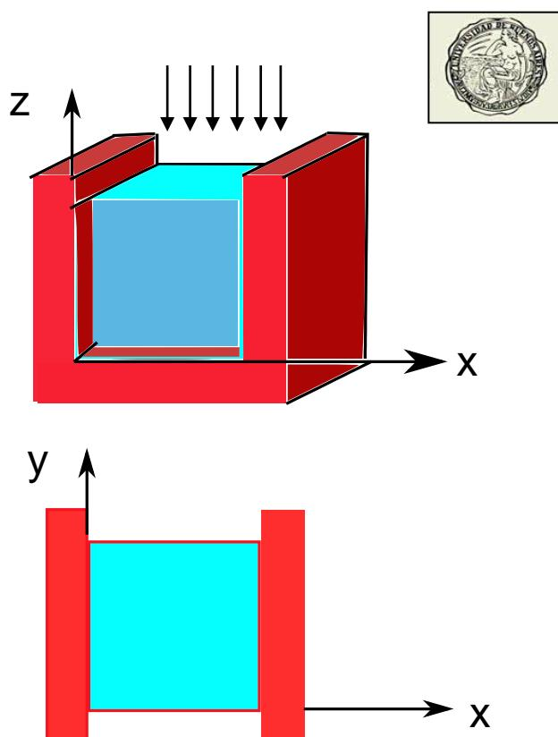
$$\varepsilon_x = \frac{\sigma_x}{E} - \mu \cancel{\frac{\sigma_y}{E}} - \mu \frac{\sigma_z}{E} = 0 \quad \rightarrow \quad \sigma_x = -\mu \cdot P_z = -0,12 \frac{kN}{cm^2}$$
