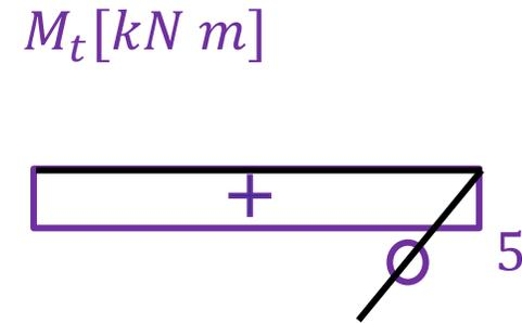
$$\eta_A = \int_L M_{se} \cdot \frac{M_{dv}}{E \cdot J} dx + \int_L Mt_{se} \cdot \frac{Mt_{dv}}{G \cdot J_t} dx = \eta_A^{M_y} + \eta_A^{M_t}$$
