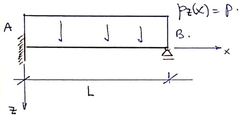
$$\left\{ \begin{array}{l} \text{IPN 200 } \gamma_{\text{acero}} = 15 \text{ kN/cm}^2 \\ E = 21.000 \text{ kN/cm}^2 \\ L = 4 \text{ m} \end{array} \right.$$
