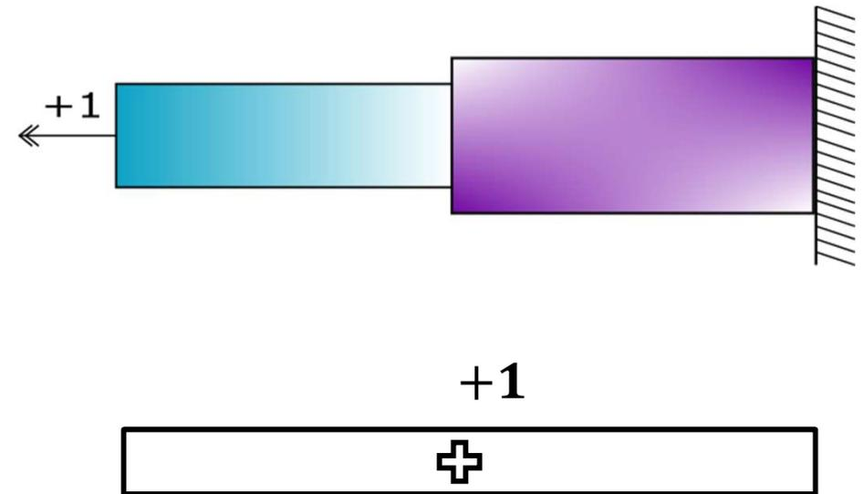
$$\theta_A^{M_t} = \int_l M_{SE} d\theta = \int_l M_{SE} \cdot \frac{M_{DV}}{G \cdot J} dx = M_{SE} \cdot \frac{M_{DV_1} \cdot L_2}{G_b \cdot J_b} = +1 \cdot \frac{-1000 \text{ kN cm} \cdot 300 \text{ cm}}{6000 \frac{\text{kN}}{\text{cm}^2} \cdot 800 \text{ cm}^4}$$
