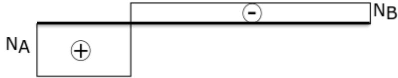
$$N_B = -P \cdot \left(1 + \frac{L_2}{L_1}\right) = -28.57 \text{ kN} \quad N_A = P + N_B = 71.43 \text{ kN}$$
