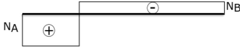
$$N_B := -P \cdot \left( \frac{L_1}{L_1 + L_2} \right) = -28.57 \text{ kN} \quad N_A := P + N_B = 71.43 \text{ kN}$$
