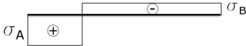
$$\sigma_A := \frac{N_A}{A} = 3.64 \frac{\text{kN}}{\text{cm}^2} \quad \sigma_B := \frac{N_B}{A} = -1.455 \frac{\text{kN}}{\text{cm}^2}$$
