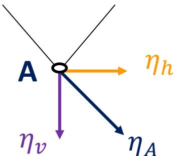
$$\begin{aligned}\eta_v &= \text{desp. vertical de } A \\ \eta_h &= \text{desp. horizontal de } A\end{aligned}$$
