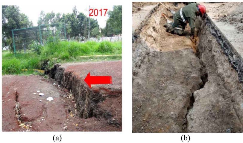
Figure 14. Soil fractures induced by (a) regional subsidence (b) hydraulic fracturing in flooding zones.
