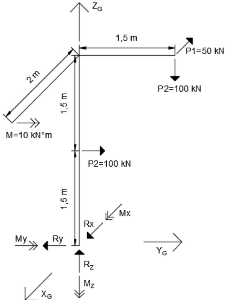
$$\sum F_x = 0 \rightarrow -50 \text{ kN} + R_x = 0 \rightarrow R_x = 50 \text{ kN}$$
