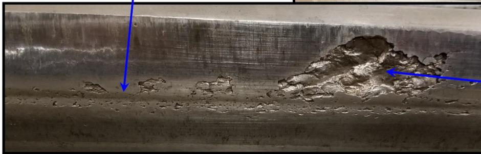
Pitting at the pitchline propagates into the addendum – spalling
