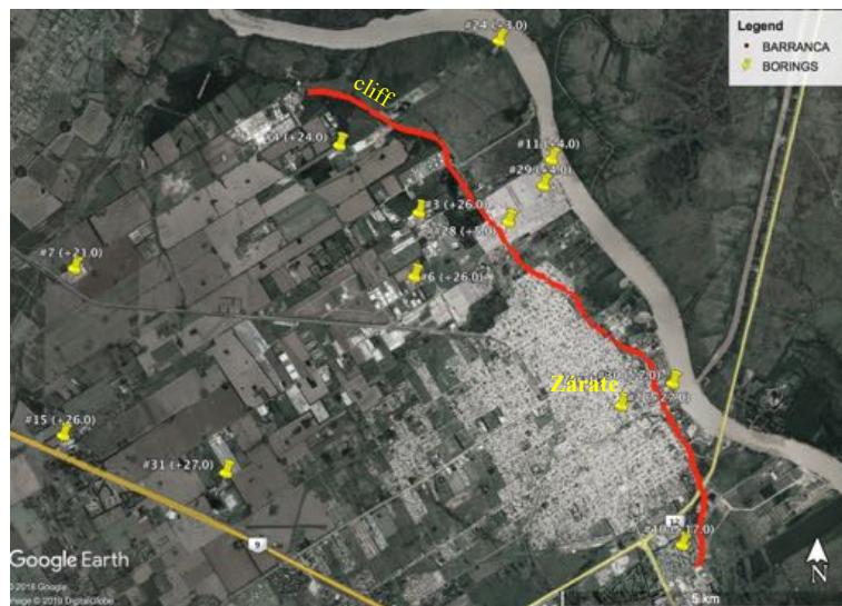
Figure 4. SPT borings on Zárate city.
