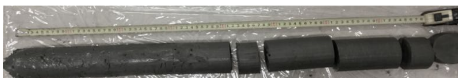
Figure 6. Sample of Postpampeano soil by fixed piston sampler.
