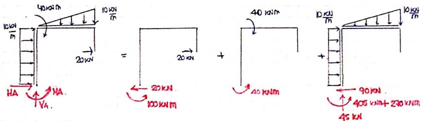
luego  $HA = 100 \text{ kNm} + 40 \text{ kNm} + 405 \text{ kNm} + 270 \text{ kNm} = \underline{\underline{815 \text{ kNm}}}$
