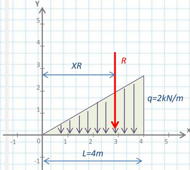
$$R = \frac{2 \frac{kN}{m} \cdot 4m}{2} = 4kN \wedge R = R1 + R2 \therefore R2 = R - R1 = 2.5kN$$
