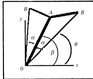
**Problem 2.35** The magnitude of the position vector  $\mathbf{r}_{BA}$  from point  $B$  to point  $A$  is 6 m and the magnitude of the position vector  $\mathbf{r}_{CA}$  from point  $C$  to point  $A$  is 4 m. What are the components of  $\mathbf{r}_{BA}$ ?
