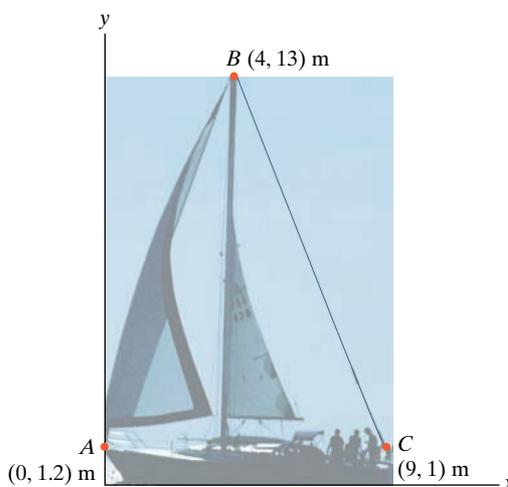
**Problem 2.108** Determine the angle  $\theta$  between the lines  $AB$  and  $AC$  (a) by using the law of cosines (see Appendix A); (b) by using the dot product.
