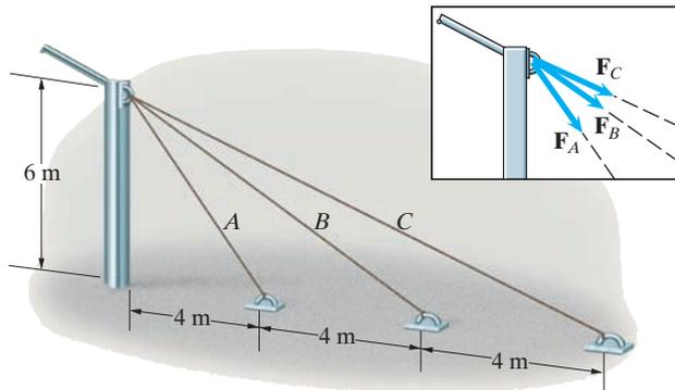
**Solution:** Use the angles and magnitudes to determine the vector components, take the sum, and solve for the unknown. The angles between each cable and the pillar are:
