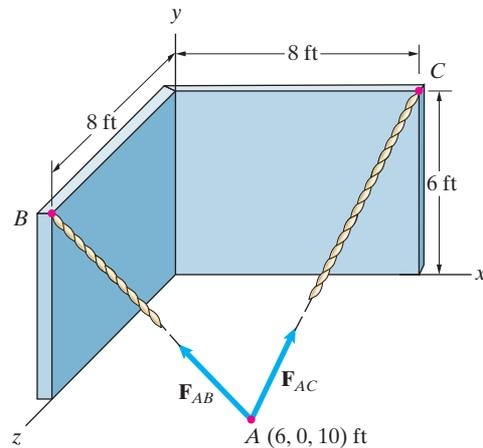
**Problem 2.92** Consider the cables and wall described in Problem 2.91. Cable  $AB$  exerts a 200-lb force  $\mathbf{F}_{AB}$  at point  $A$  that is directed along the line from  $A$  to  $B$ . The cable  $AC$  exerts a 100-lb force  $\mathbf{F}_{AC}$  at point  $A$  that is directed along the line from  $A$  to  $C$ . Determine the magnitude of the total force exerted at point  $A$  by the two cables.
