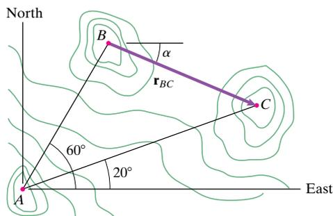
**Solution:** Draw the vectors accurately and then measure the unknown magnitude and angle.
