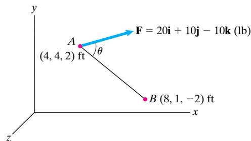
**Problem 2.152** Determine the scalar components of a unit vector parallel to line  $AB$  that points from  $A$  toward  $B$ .
