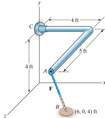
**Solution:** We need to determine the force  $\mathbf{F}$  in terms of its components. The vector from  $A$  to  $B$  is used to define  $\mathbf{F}$ .
