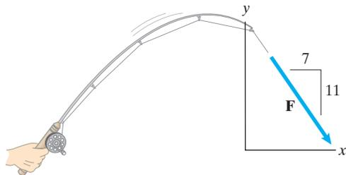
**Solution:** We can use similar triangles to determine the components of  $\mathbf{F}$ .
