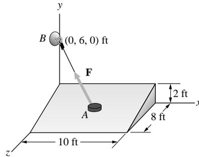
**Solution:** Consider a line on the sloped surface from  $A$  perpendicular to the surface. (see the diagram above) By SIMILAR triangles we see that one such vector is  $\mathbf{r}_N = 8\mathbf{j} + 2\mathbf{k}$ . Let us find the component of  $\mathbf{F}$  parallel to this line.
