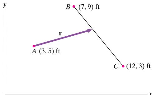
**Solution:** Determine the perpendicular vector to the line  $BC$  from point  $A$ , and then use this perpendicular to determine the angular orientation of the vector  $\mathbf{r}$ . The vectors are
