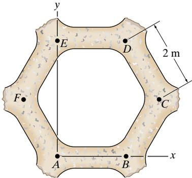
**Solution:** Use the  $xy$  coordinate system shown and find the locations of  $C$  and  $F$  in those coordinates. The coordinates of the points in this system are the scalar components of the vectors  $\mathbf{r}_{AC}$  and  $\mathbf{r}_{AF}$ . For  $\mathbf{r}_{AC}$ , we have
