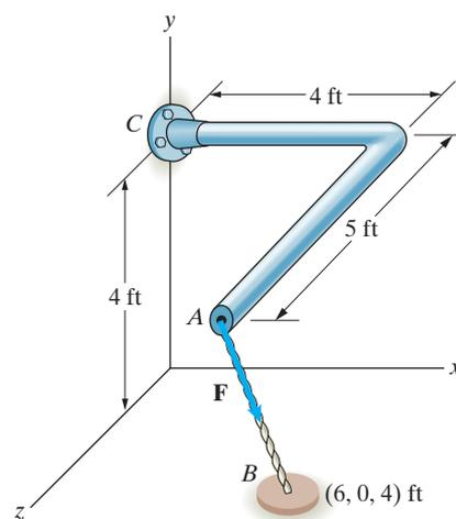
**Problem 2.127** The two segments of the L-shaped bar are parallel to the  $x$  and  $z$  axes. The rope  $AB$  exerts a force of magnitude  $|\mathbf{F}| = 500$  lb on the bar at  $A$ . Determine the cross product  $\mathbf{r}_{CB} \times \mathbf{F}$ , where  $\mathbf{r}_{CB}$  is the position vector from point  $C$  to point  $B$ . Compare your answers to the answer to Problem 2.126.
