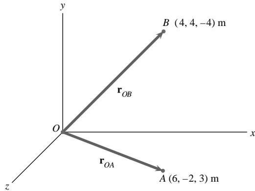
**Problem 2.135** For the points  $O$ ,  $A$ , and  $B$  in Problem 2.134, use the cross product to determine the length of the shortest straight line from point  $B$  to the straight line that passes through points  $O$  and  $A$ .
