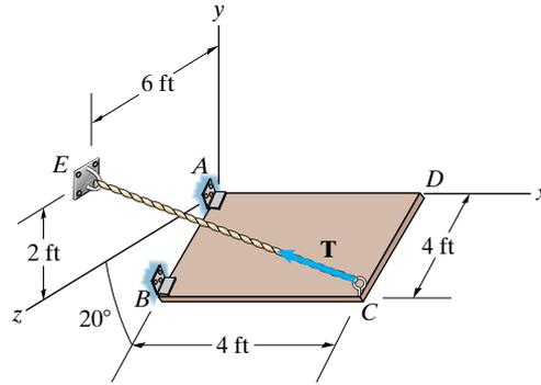
**Solution:** Find the unit vector  $\mathbf{e}_{CE}$  and multiply it times the magnitude of the force to get the vector in component form,
