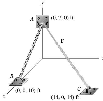
**Problem 2.115** Consider the cables  $AB$  and  $AC$  shown in Problem 2.114. Let  $\mathbf{r}_{AB}$  be the position vector from point  $A$  to point  $B$ . Determine the vector component of  $\mathbf{r}_{AB}$  parallel to the cable  $AC$ .
