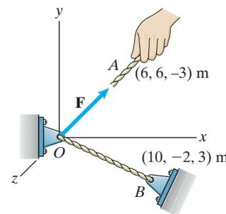
**Problem 2.112** The person exerts a force  $\mathbf{F} = 60\mathbf{i} - 40\mathbf{j}$  (N) on the handle of the exercise machine. Use Eq. (2.26) to determine the vector component of  $\mathbf{F}$  that is parallel to the line from the origin  $O$  to where the person grips the handle.
