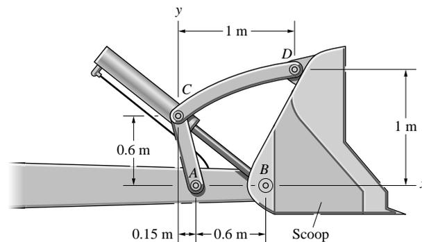
**Problem 2.40** The hydraulic actuator  $BC$  in Problem 2.39 exerts a 1.2-kN force  $\mathbf{F}$  on the joint at  $C$  that is parallel to the actuator and points from  $B$  toward  $C$ . Determine the components of  $\mathbf{F}$ .
