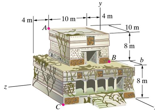
**Solution:** We have the coordinates  $B(10 \text{ m}, 8 \text{ m}, 4 \text{ m})$ ,  $C(10 \text{ m} + b, 0, 18 \text{ m})$ .
