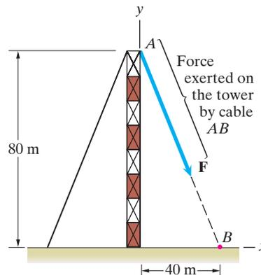
**Problem 2.32** Determine the position vector  $\mathbf{r}_{AB}$  in terms of its components if (a)  $\theta = 30^\circ$ , (b)  $\theta = 225^\circ$ .
