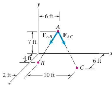
**Solution:** The new coordinates of point  $A$  are  $(6, 8, 0)$  ft. The position vectors are
