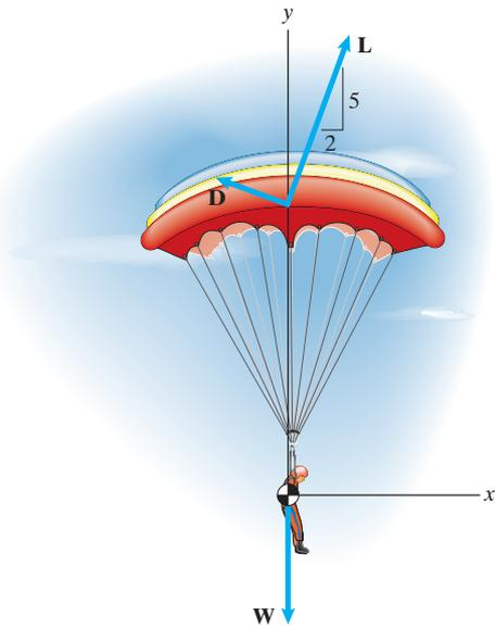
**Solution:** Let  $L$  and  $D$  be the magnitudes of the lift and drag forces. We can use similar triangles to express the vectors  $\mathbf{L}$  and  $\mathbf{D}$  in terms of components. Then the sum of the forces is zero. Breaking into components we have
