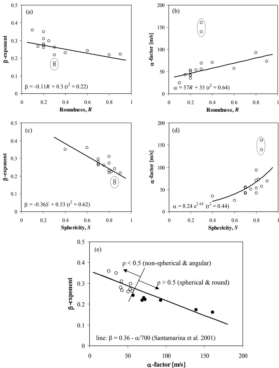
**Fig. 8.** The effect of particle shape on small-strain shear wave velocity (data in Table A1). The two encircled points in Fig. 8(a~d) correspond to Ponte Vedra and Jekyll Island sands which contain a high percentage of crushed shells.
