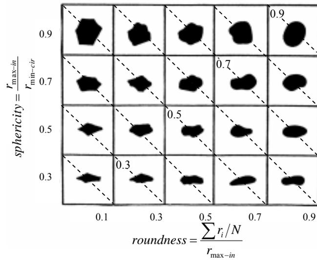
**Fig. 1.** Sphericity  $S$  and roundness  $R$  chart. Diagonal dotted lines correspond to constant particle regularity  $\rho=(R+S)/2$  (modified from Krumbein and Sloss 1963).
