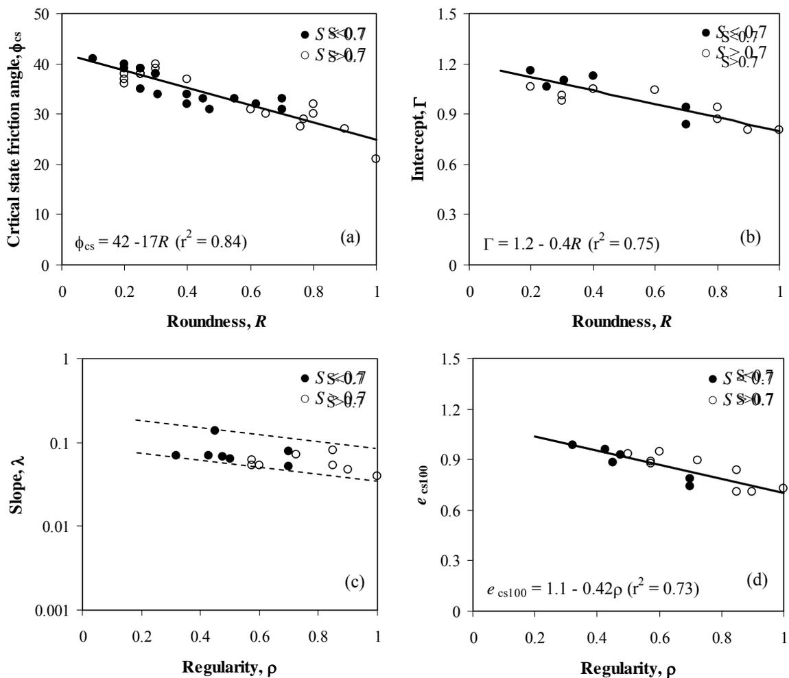
**Fig. 10.** The effect of particle shape on critical state parameters (data in Table A1).
