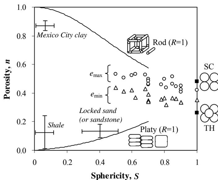
**Fig. 6.** Variation of porosity with sphericity. Trends: geometric analysis based on the extreme packings shown in the figure (particles remain round  $R=1$ ). Data points: natural sands (this study - Table A1). Extreme values at  $S=1$  correspond to simple cubic SC packing, tetrahedral TH packing, and experimental data with glass beads. Ranges: from published studies.
