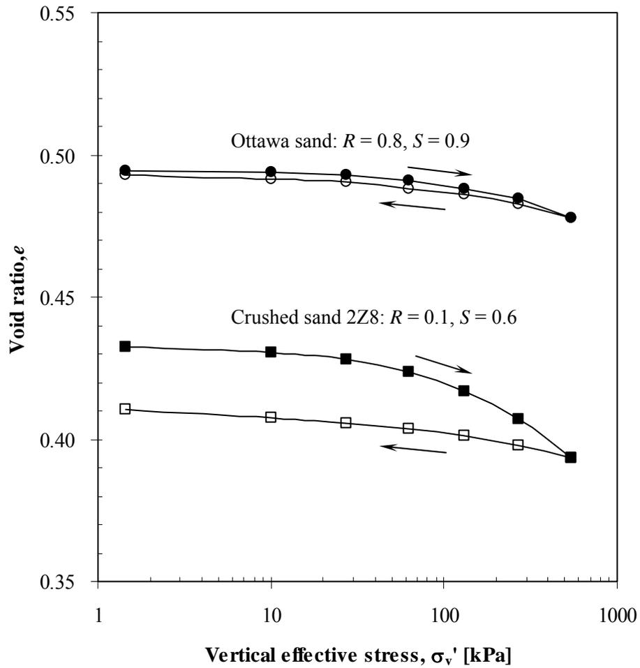
**Fig. 3.** The variation of void ratio with vertical effective stress during zero-lateral strain loading (additional properties for these sands can be found in Table A1).
