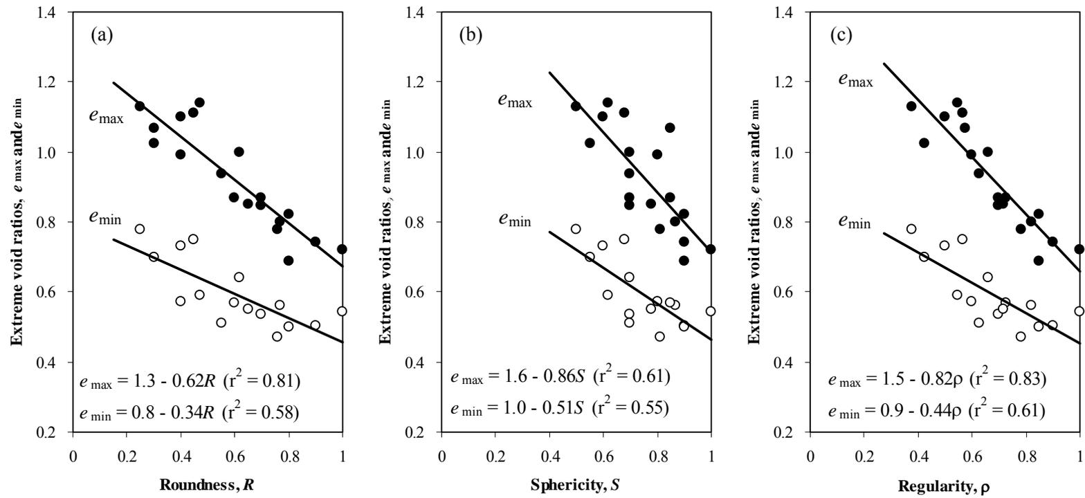
**Fig. 5.** Effect of particle shape on extreme void ratios (natural sands with  $C_u \leq 2.5$  - Data in Table A1).
