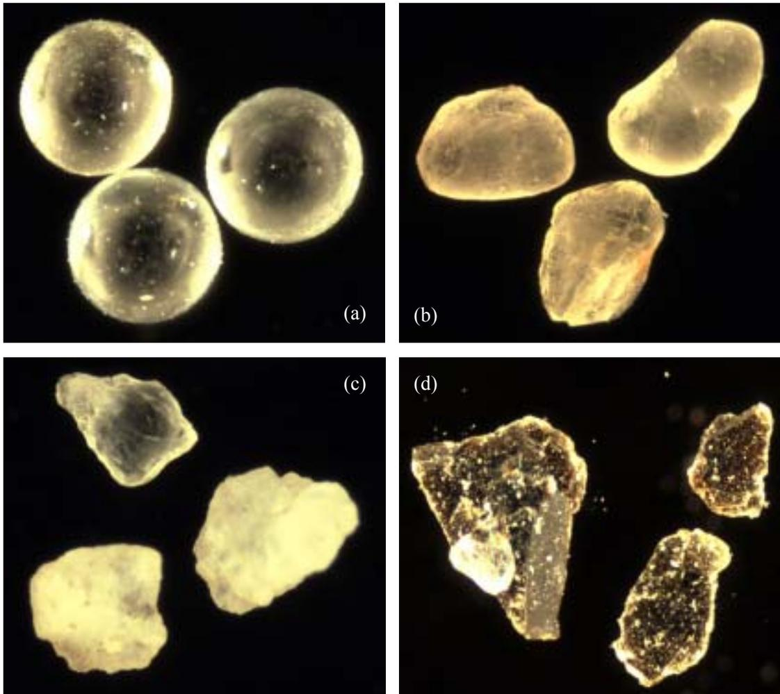
**Fig. 2.** Microphotographs of typical grains tested in this study. (a) Glass beads  $D_{50} = 0.15$  mm. (b) Ottawa sand  $D_{50} = 0.60$  mm. (c) Ticino sand  $D_{50} = 0.33$  mm. (d) Fine fraction of crushed sands  $D \approx 0.08$  mm.
