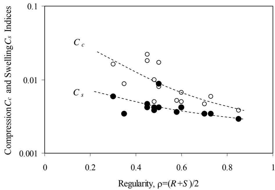
**Fig. 9.** The effect of particle shape on zero-lateral strain oedometric stiffness during compression and expansion (data in Table A1).
