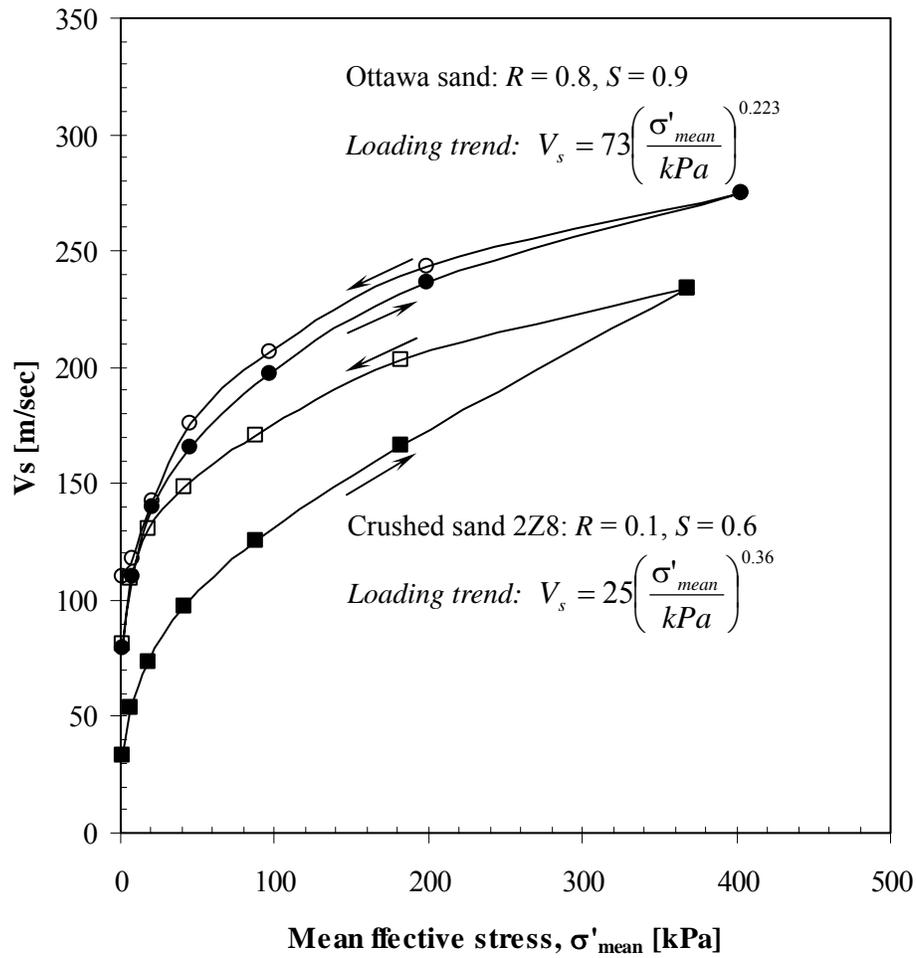
**Fig. 7.** Variation of shear wave velocity with effective confining stress (Refer to Fig. 4 – additional properties for these sands can be found in Table A1).
