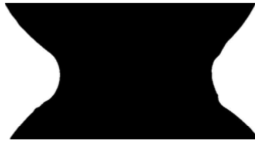
Figure 5. Evolution of unsaturation – Pendular regime. The lower spherical glass bead ( d=2\text{mm} ) is being held by the meniscus. Top sequence: de-ionized water. Lower sequence: water has salt in solution, salts eventually precipitate rendering inter-particle cementation (Gathered with D. Fratta).
