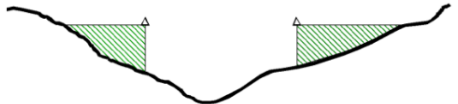
C. Portion of cross sections 2 & 3 that is ineffective for low flow
