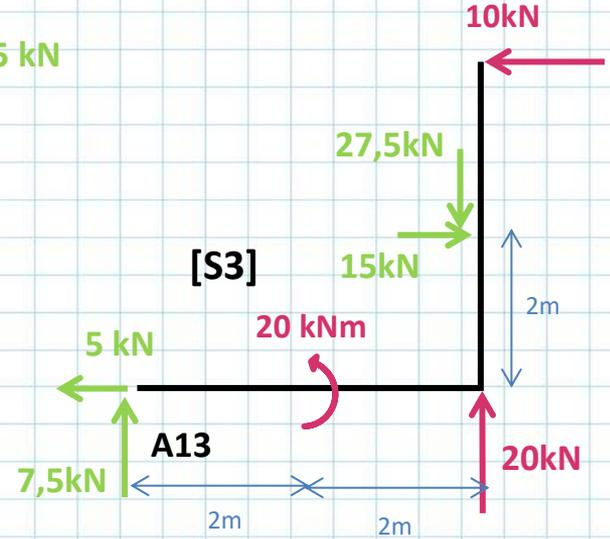
$$\Sigma F_{xS3} := 15 \text{ kN} - 10 \text{ kN} - 5 \text{ kN} = 0 \text{ kN}$$
