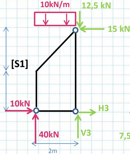
$$\Sigma F_{xS1} \quad H_3 + 10 \text{ kN} - 15 \text{ kN} = 0 \xrightarrow{\text{solve, } H_3} 5 \cdot \text{kN}$$
