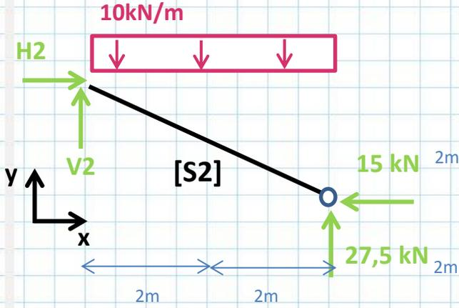
$$\Sigma F_{xS2} \quad H_2 - 15 \text{ kN} = 0 \xrightarrow{\text{solve, } H_2} 15 \cdot \text{kN}$$
