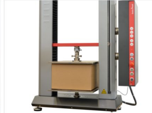
Compression test on packaging
