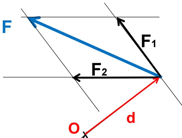
$$\begin{aligned}\bar{M}_{O,F} &= \bar{d} \times \bar{F}_1 + \bar{d} \times \bar{F}_2 \\ \bar{M}_{O,F} &= \bar{d} \times (\bar{F}_1 + \bar{F}_2) \\ \bar{M}_{O,F} &= \bar{d} \times \bar{F}\end{aligned}$$
