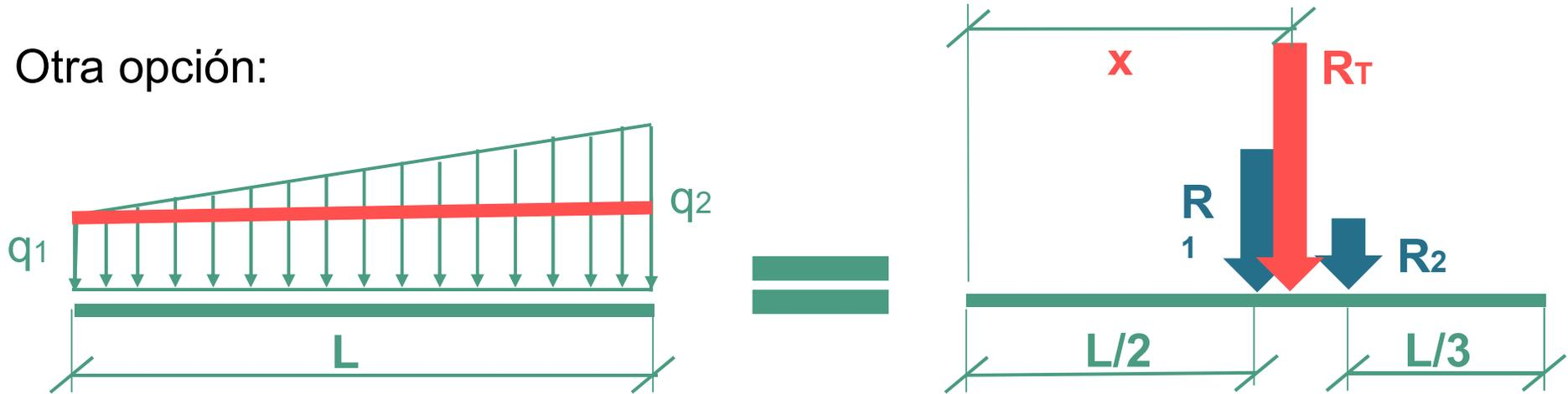
$$R_1 = q_1 \times L \qquad R_2 = \frac{(q_2 - q_1) \times L}{2}$$
