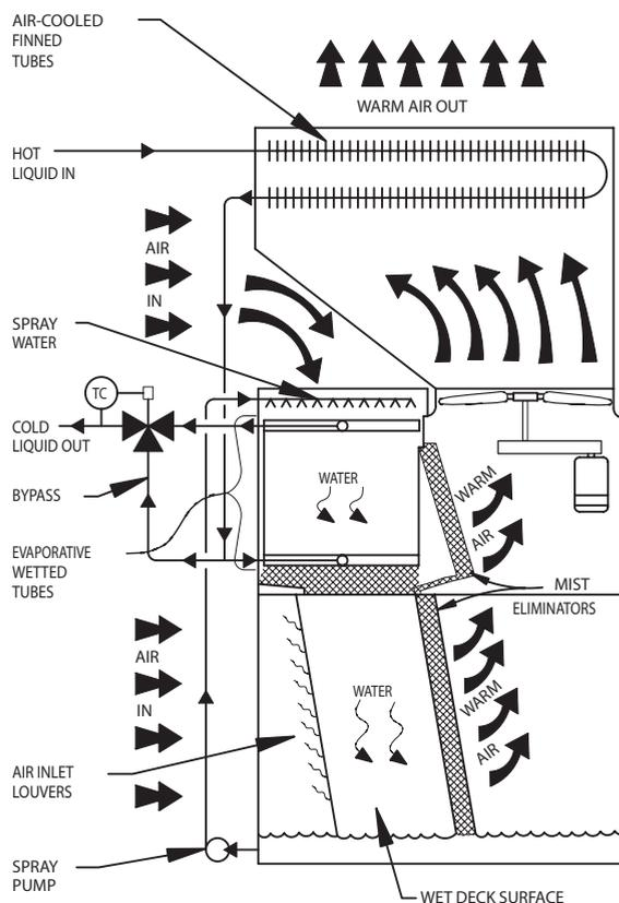
FIG. 12-8p As seasonal ambient temperatures drop, the "wet-dry" configuration for a WSAC progressively shifts the cooling load from evaporative to convective cooling.
