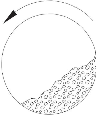
FIG. 12-27a Horizontal moving bed.
