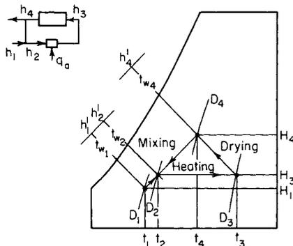
FIG. 12-6f Drying process with recirculation.
