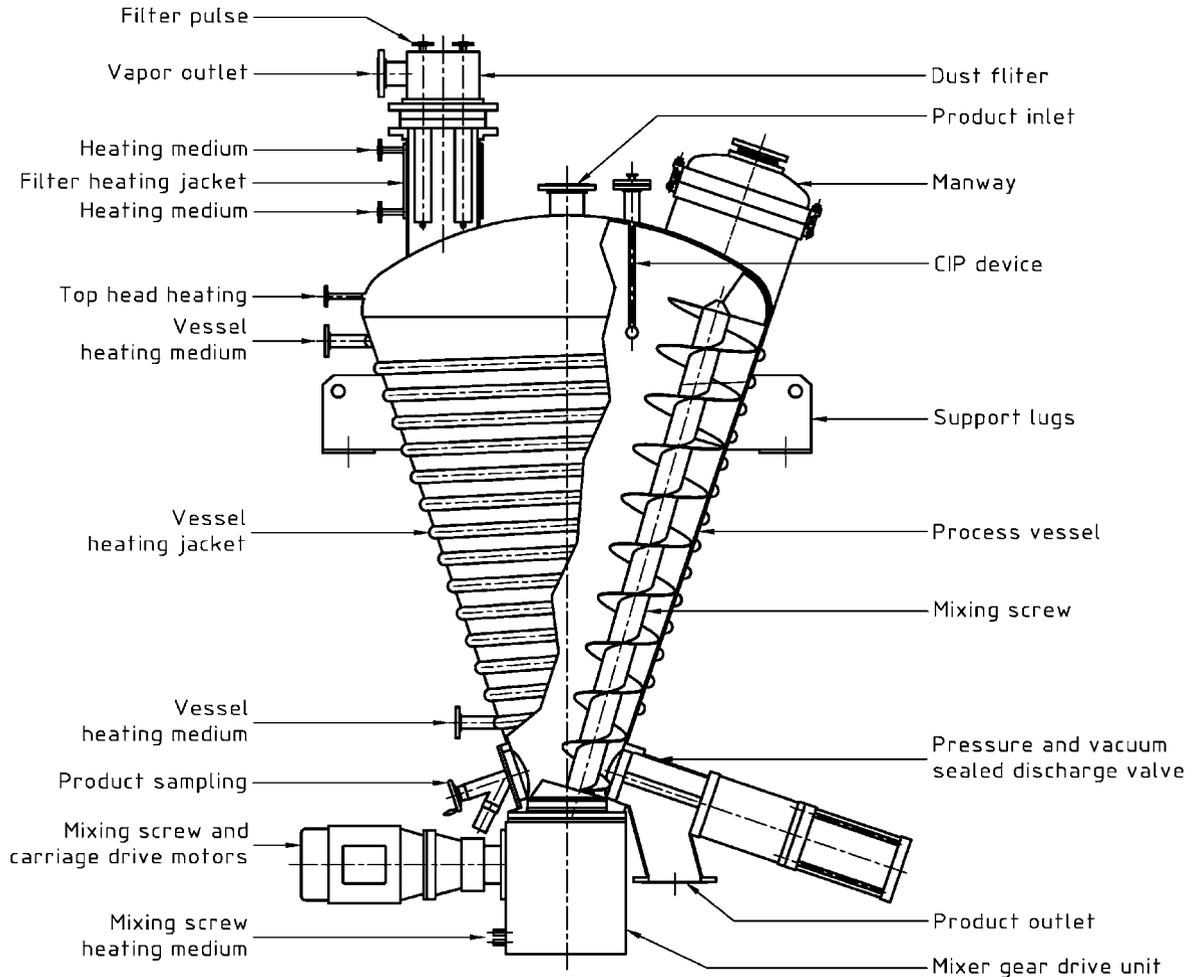
FIG. 12-53 Bottom-drive conical mixer dryer. (Krauss Maffei.)
