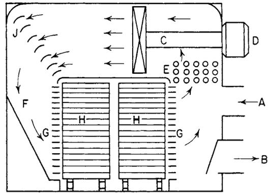
**FIG. 12-44** Double-truck tray dryer. (A) Air inlet duct. (B) Air exhaust duct with damper. (C) Adjustable-pitch fan 1 to 15 hp. (D) Fan motor. (E) Fin heaters. (F) Plenum chamber. (G) Adjustable air blast nozzles. (H) Trucks and trays. (J) Turning vanes.
