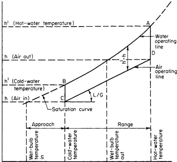
FIG. 12-8a Cooling-tower process heat balance. (Marley Co.)
