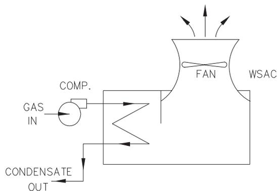
FIG. 12-8l WSAC configuration for condensing a compressed gas. A lower condensing pressure reduces compressor operating horsepower.
