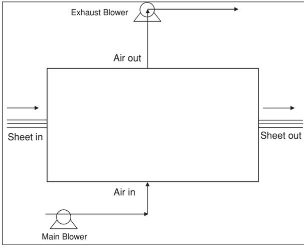
FIG. 12-10 Overall mass and energy balance diagram.
