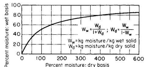
FIG. 12-9 Relationship between wet-weight and dry-weight bases.
