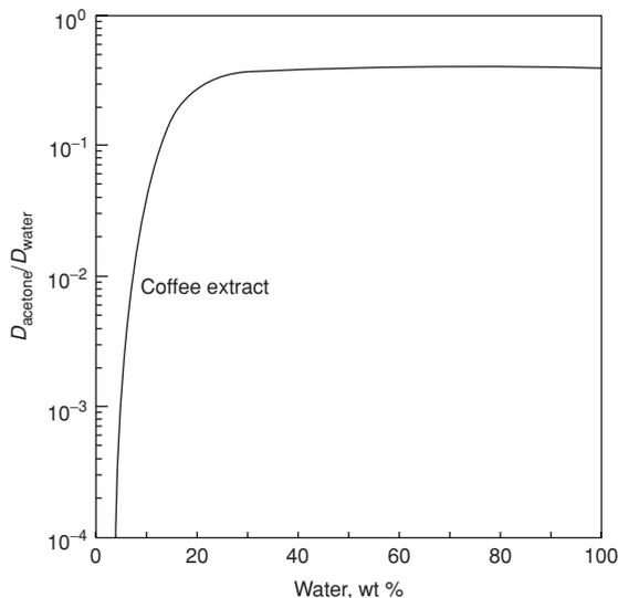
**FIG. 12-22** The ratio of the diffusion coefficients of acetone to water in instant coffee as a function of moisture content (taken from Thijssen et al., *De Ingenieur*, JRG, 80, Nr. 47 (1968)]. Acetone has a much higher vapor pressure than water, but is selectively retained in coffee during drying.
