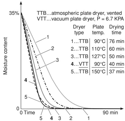
FIG. 12-48 Plate dryer drying curves demonstrating impact of elevated temperature and/or operation under vacuum. (Krauss Maffei.)
