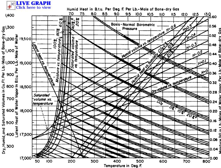
FIG. 12-4 Grosvenor psychrometric chart for air and flue gases at high temperatures, molar units [Hatta, Chem. Metall. Eng., 37:64 (1930)].
