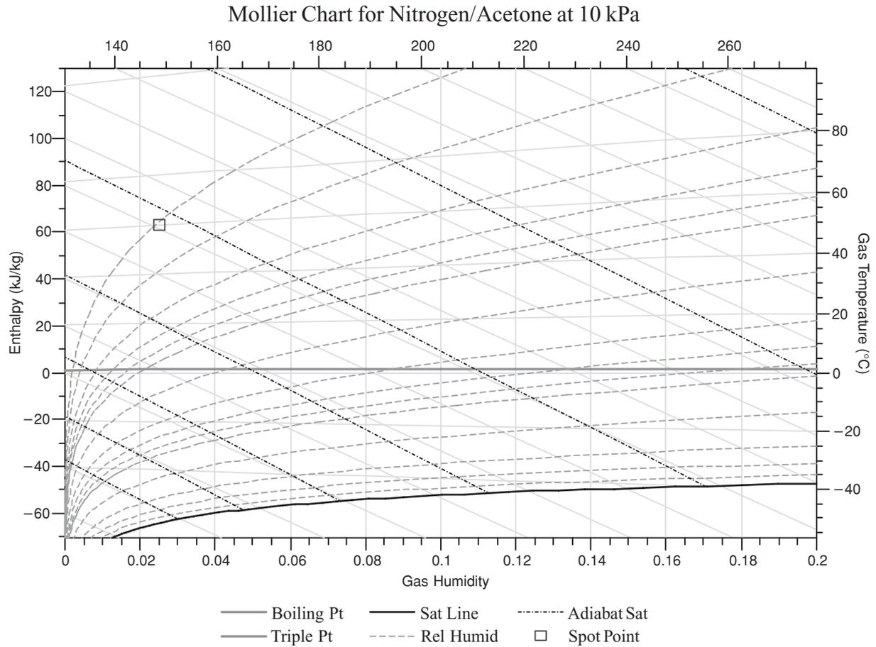
**FIG. 12-7** Mollier psychrometric chart (from PSYCHIC software program) showing determination of adiabatic saturation temperature plots humidity (abscissa) against enthalpy (lines sloping diagonally from top left to bottom right). (Courtesy AspenTech.)
