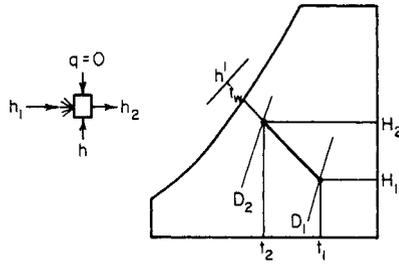
FIG. 12-6c Spray or evaporative cooling.
