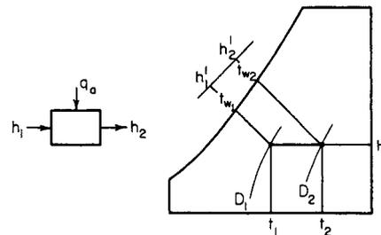
FIG. 12-6b Heating process
