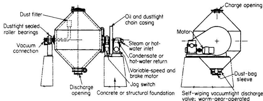
FIG. 12-55 Rotating (double-cone) vacuum dryer. (Stokes Vacuum, Inc.)
