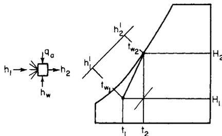
FIG. 12-6e Cooling tower.
