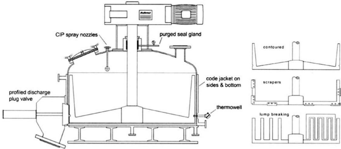
FIG. 12-52 Vertical pan dryer. (Bufllovak Inc.)
