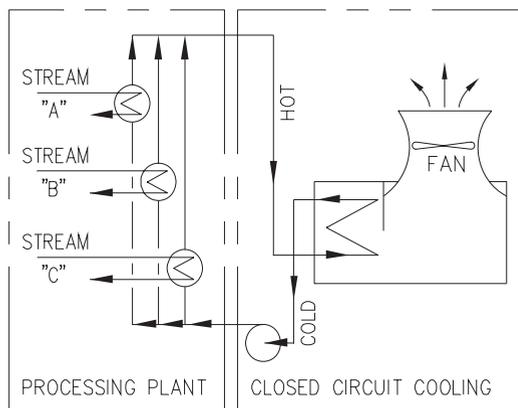
FIG. 12-8o WSAC configuration with no direct fluid contact.
