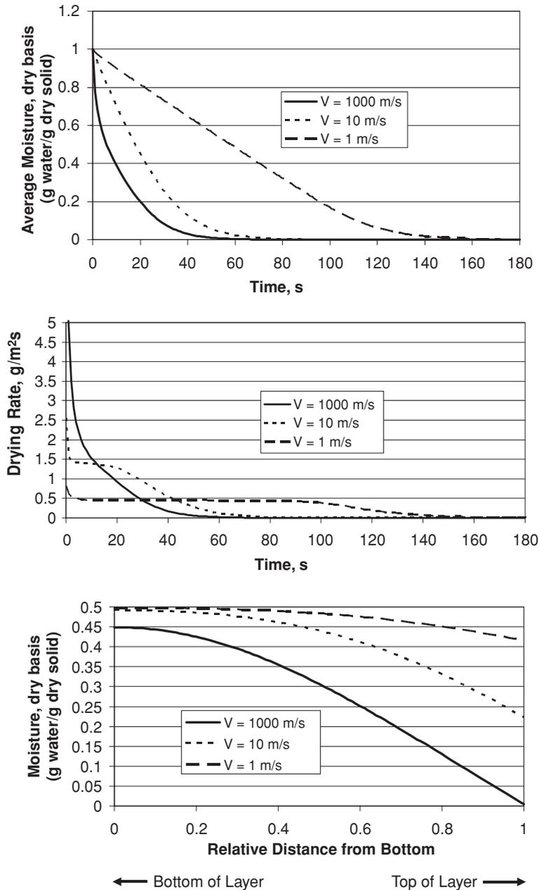
FIG. 12-16 Simulation results for thin layer drying example.
