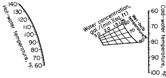
**FIG. 12-8c** Sizing chart for a counterflow induced-draft cooling tower. For induced-draft towers with (1) an upspray distributing system with 24 ft of fill or (2) a flume-type distributing system and 32 ft of fill. The chart will give approximations for towers of any height. (Ecodyne Corp.)
