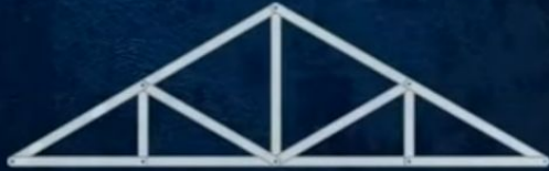
Howe roof truss
