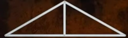
King Post roof truss
