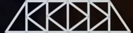
K bridge truss
