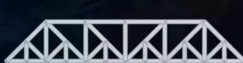
Baltimore bridge truss
