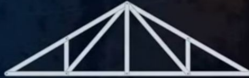
Pratt roof truss
