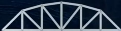
Parker bridge truss
