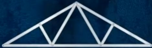
Fink roof truss
