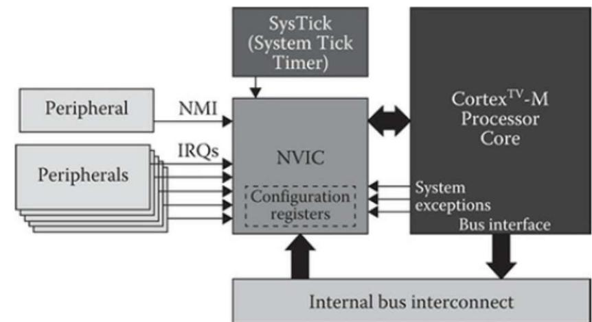
Figure 6-1 NVIC block diagram.
