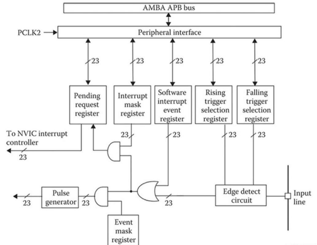
Figure 6-3 EXTI block diagram.
