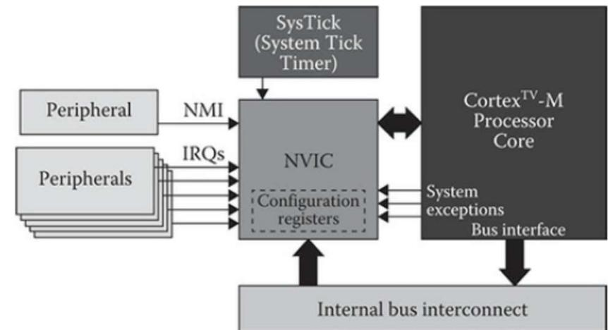
Figure 6-1 NVIC block diagram.
