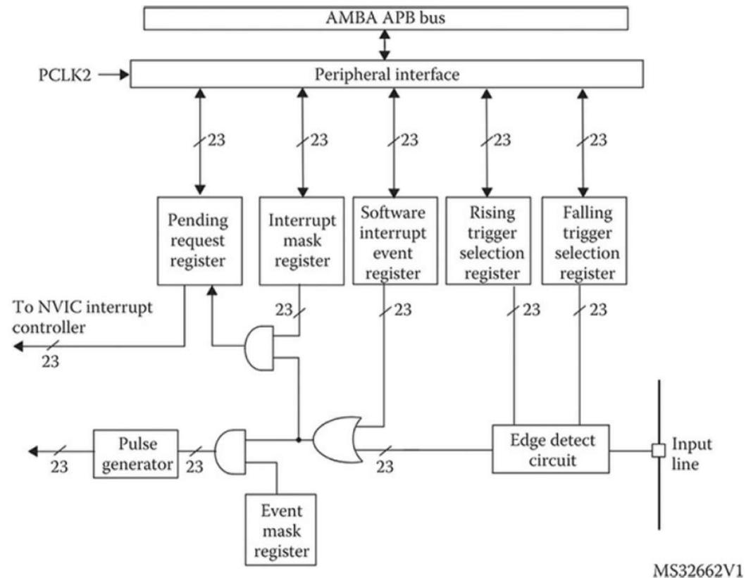
Figure 6-3 EXTI block diagram.
