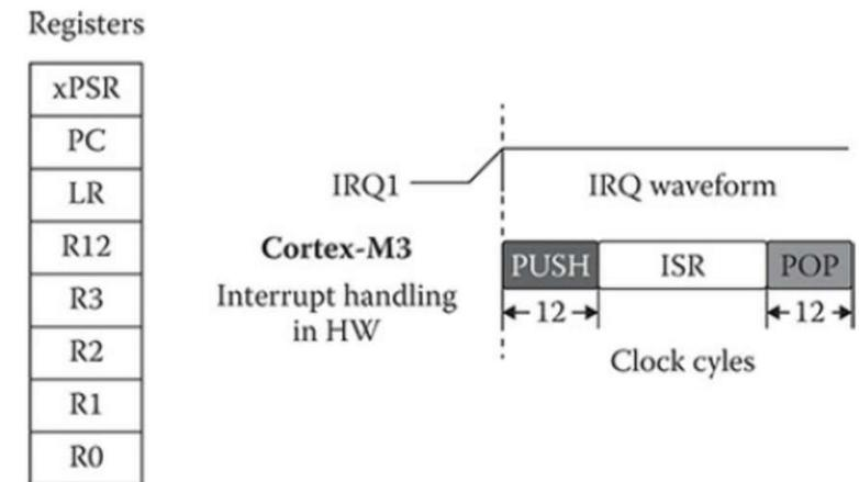
Figure 6-2 Interrupt processing sequence.
