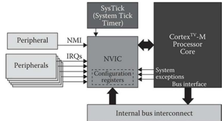
Figure 6-1 NVIC block diagram.
