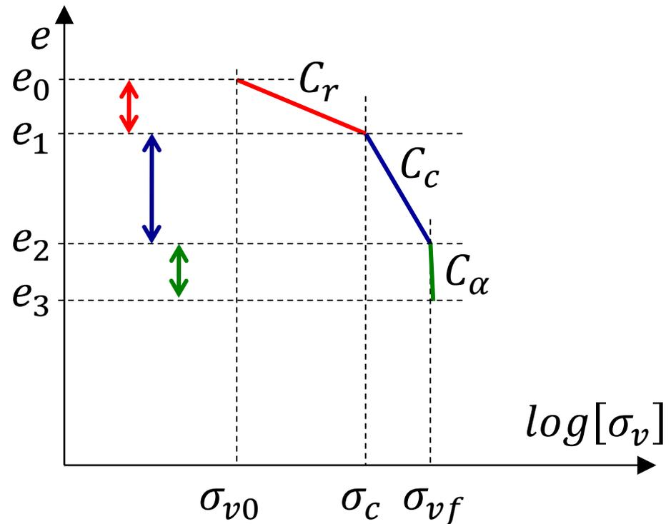
$$\Delta h = \left( \frac{C_r}{1 + e_0} \log \left[ \frac{\sigma_c}{\sigma_{v0}} \right] + \frac{C_c}{1 + e_1} \log \left[ \frac{\sigma_{vf}}{\sigma_c} \right] + \frac{C_\alpha}{1 + e_2} \log \left[ \frac{t}{t_p} \right] \right) h$$
