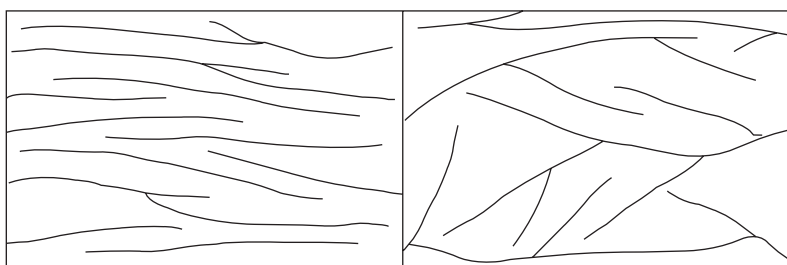
12.8 Polyethylene homopolymer in its two main forms: high density polyethylene (HDPE) on the left, and low density polyethylene (LDPE) on the right.
