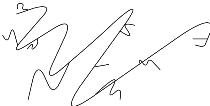
12.6 Branched polymer showing short and long chain branching (e.g. LDPE).
