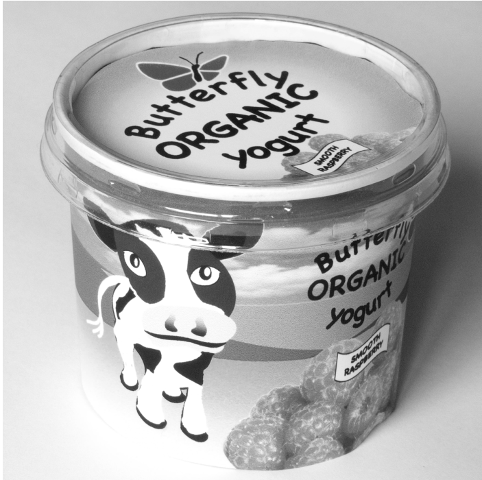
18.11 Mock-up of paperboard yoghurt pot. The rough graphics from the previous figure were converted to an arc shape, printed and simply applied to an ice cream carton – a quick and effective way of creating a mock-up.
