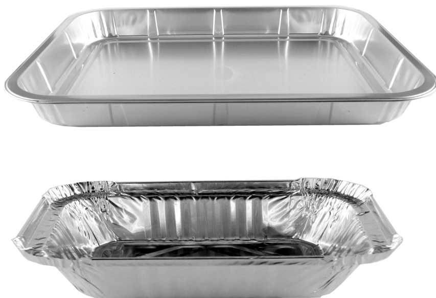
9.6. Examples of a smooth wall heavy gauge deep drawn aluminium container (above) and a wrinkle wall narrow gauge shallow drawn aluminium container (below).
